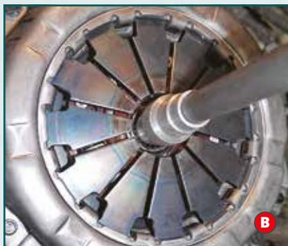
Choose a suitable-sized adapter that fits to the center of flywheel, and connect to spindle. Insert the cone adapter through the spindle, and align the flywheel with clutch and pressure plate.
