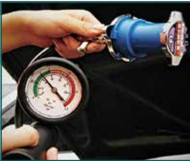
Connect the original radiator cap to one side of the connector, and a pressure test cap on the other side (Fig. 2). Pump pressure to the specified pressure on the cap. When pumping pressure under the specified pressure, check if the gauge reading drops. If it does, there could be leaks in the radiator cap. When pumping pressure above the specified pressure, check if the radiator cap has the ability to release pressure. If it does not, the cap should be replaced.
