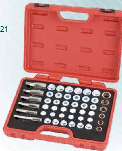
Designed for replacing the damaged oil drain nuts by using a tap to enlarge the stripped drain plug hole for fitting new nuts with bigger sizes.
