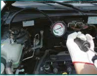
Choose a suitable adapter and screw it onto the radiator filler neck. Connect the pressure tester to the adapter. Pump pressure to the range between 10 and 15 psi (Fig. 1). Check if the gauge reading moves. If it does, there could be some leaks in the cooling system.
