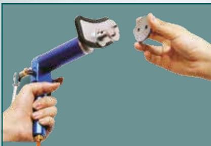
**Step 3:** Press operation button (D) and rotate the lever (C) to push the piston backward.
