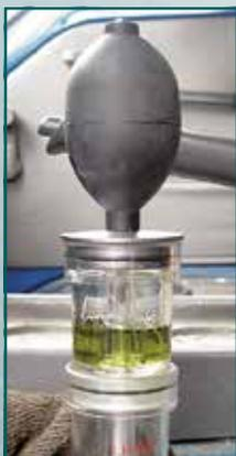
If exhaust gas presents in cooling system, the colour of test liquid turn from blue to green or yellow when CO<sub>2</sub> is detected in tester fluid (Fig. 2)
